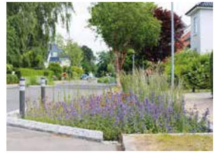
BIO-RETENTION SYSTEM FOR SURFACE RUN-OFF AT LANGELINIE, ODENSE – PHOTO BY VSC DENMARK
